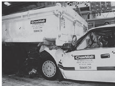
The cushioning effect of Truck Mounted Attenuators (TMAs) protects drivers and vehicles in the event of a crash.
